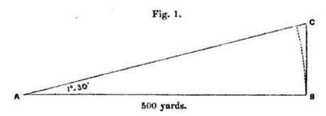
**A** being the point from which the shot started and **B** the spot where it pitched; then after leaving **A** in the direction **A C**, at an angle of 1 degree 30 minutes to the horizon, if uninfluenced by gravity, it would after traversing 500 yards reach the point **C**.
